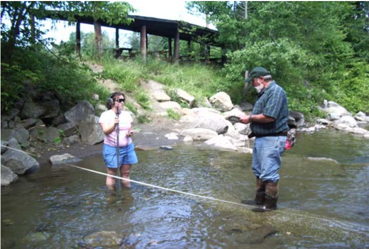
Volunteers measure stream flow as part of the water quality monitoring program in the Inner Winooski.
