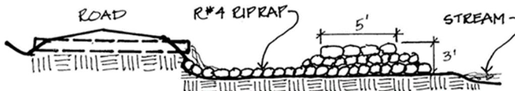
Figure 32: Plunge Pool – Section A-A View
