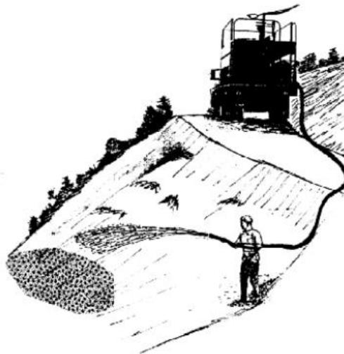
Figure 34: Hydroseeder attached to truck
