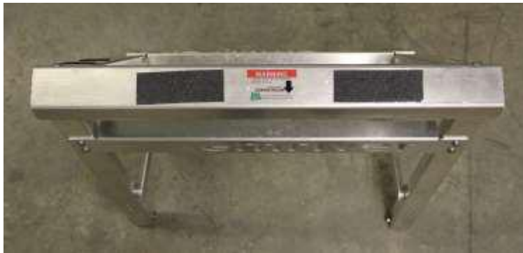
Figure 4. Labels on the supports indicate proper orientation, with the shorter support at the downstream end.
