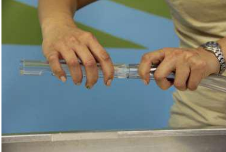
Figure 12. Insert the flow outlet into the tubing.
