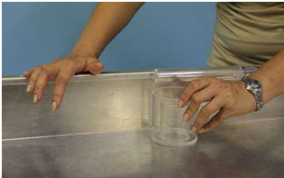
Figure 15. Place the EDU beneath the flow outlet.
