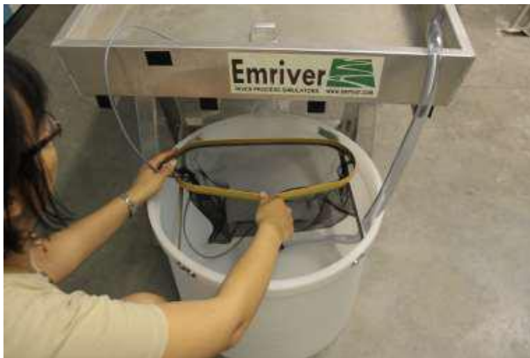
Figure 11. Place the sediment trap on the aluminum struts in the reservoir.
