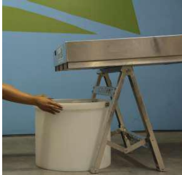
Figure 9. Place the reservoir beneath the support at the downstream end.
