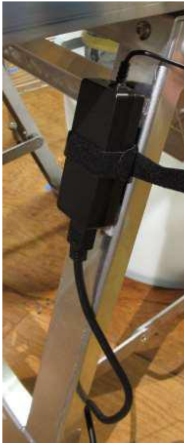
Figure 2. Power supply included with the Emriver Em2 model, shown attached to the downstream support.
