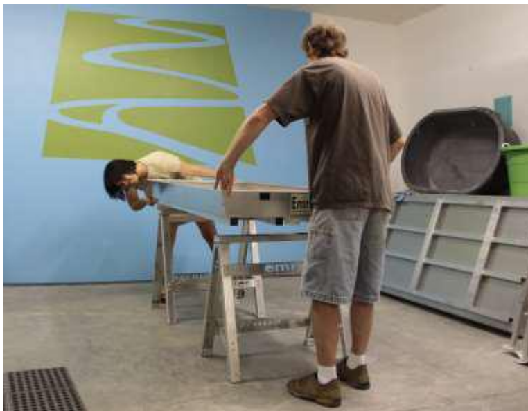
Figure 8. Check to ensure that the support ribs on the box rest on the supports properly.
