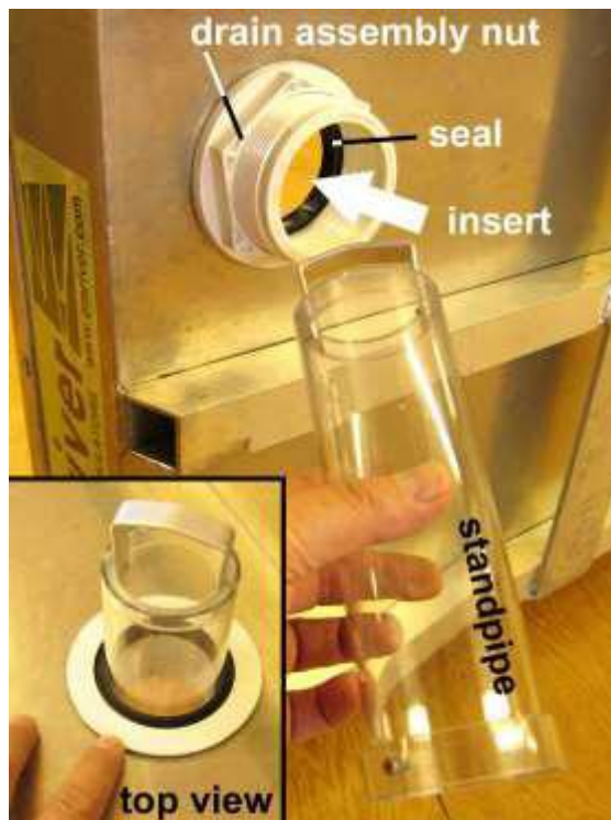
Figure 5. Insert the standpipe from the underside of the box to avoid damage to the seal. The standpipe will move much easier when the seal is wet. Never attempt to install the standpipe from the top of the box.
