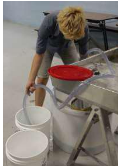
Figure 23. Place the tubing so that it drains into a smaller, separate container if there is no drainage area nearby. Turn on the pump to move water out of the reservoir.
