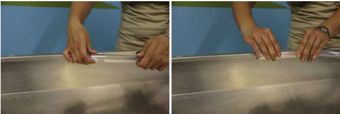
Figure 13. Align the mushroom fasteners on the flow outlet with those on the inside of the box at the upstream end. Snap the fasteners together to secure the outlet to the box.
