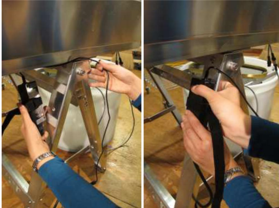
Figure 17. Attach the brick power supply to the leg of the downstream support.
