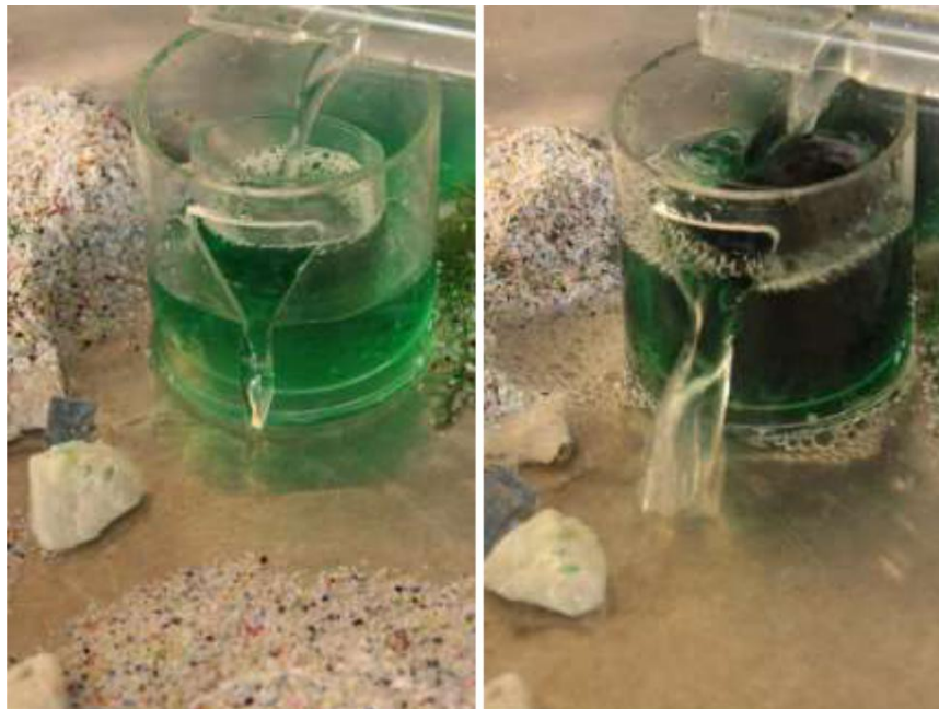
Figure 24. Low flow (left) and high flow (right) as it appears when looking at the EDU.
