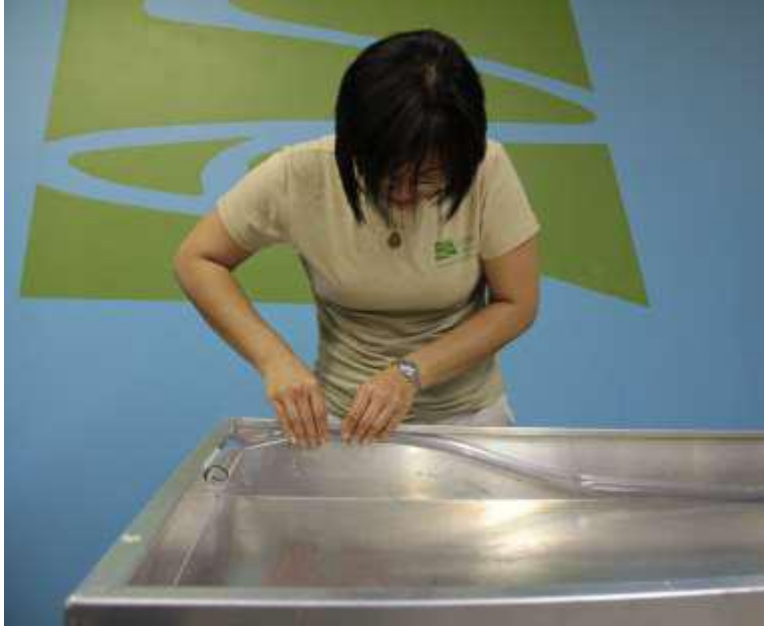
Figure 14. Tuck the tubing beneath the lip on the inside of the box.
