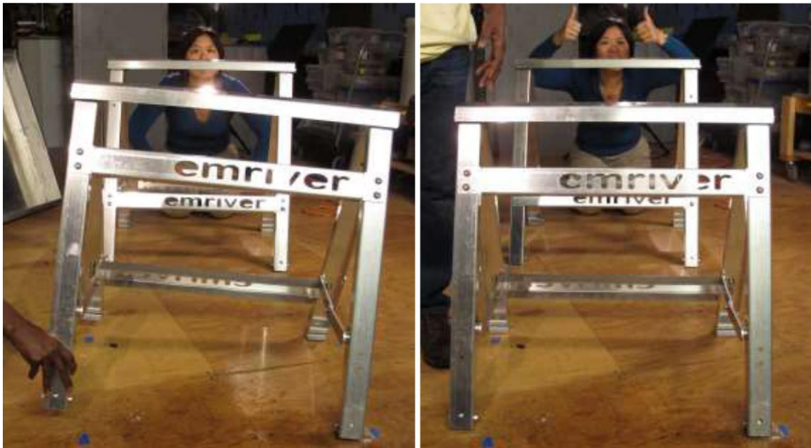
Figure 3. Incorrect (left) and correct (right) support alignment. Crossbars must be both level and parallel when viewed as shown.
