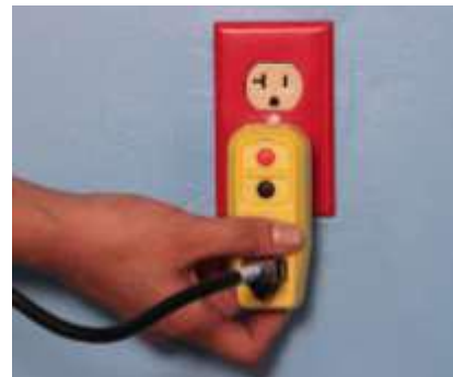
Figure 18. Always connect the power cord to the GFCI. Never plug the model's power supply directly into a wall outlet.
