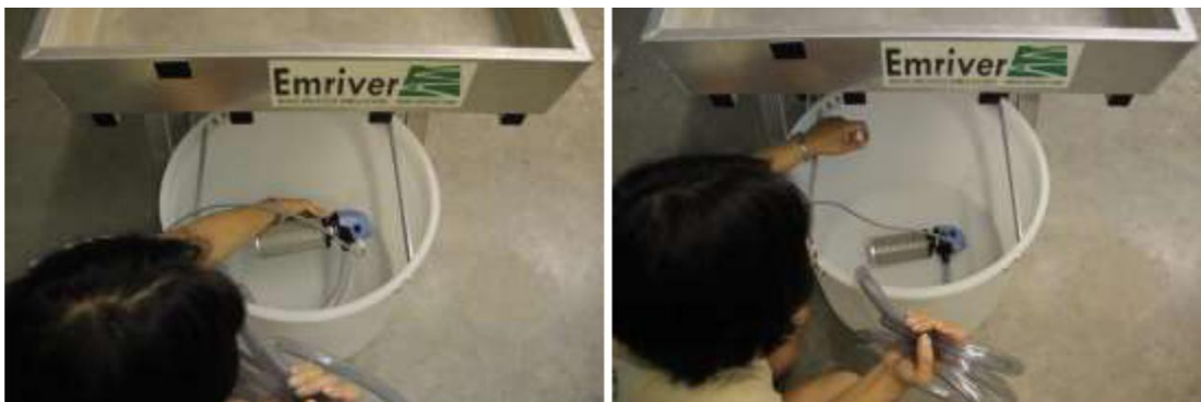
Figure 10. Place the pump in the bottom of the reservoir, lying on its side.
